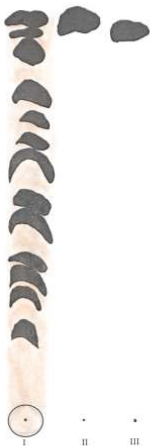
fig. 1. thin layer chromatography of the diethylether fraction of the water-ethanol extract of the stem (I) individual acetovanillone (II) and acetosyringone (III). System chloroform: methanol (80:20). Revealing substance – diazotisation sulphanilic acid.
